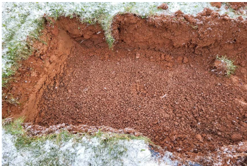
15. Looking at TP2, pea gravel observed in the shallow test pit.
