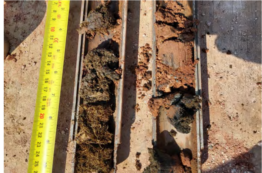
14. High amounts of organic material observed in MW23-03.
