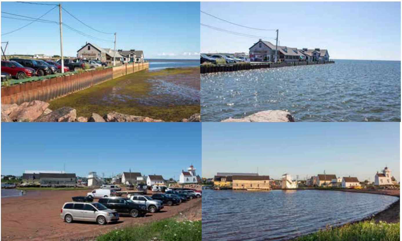
Figure 17. Low and high tide comparisons. The tidal range on the south shore at Victoria (top) can be over 2.8 m, where as the tidal range on the north shore near North Rustico is only about 1.1 m (bottom). (D. Jardine, 2023)
