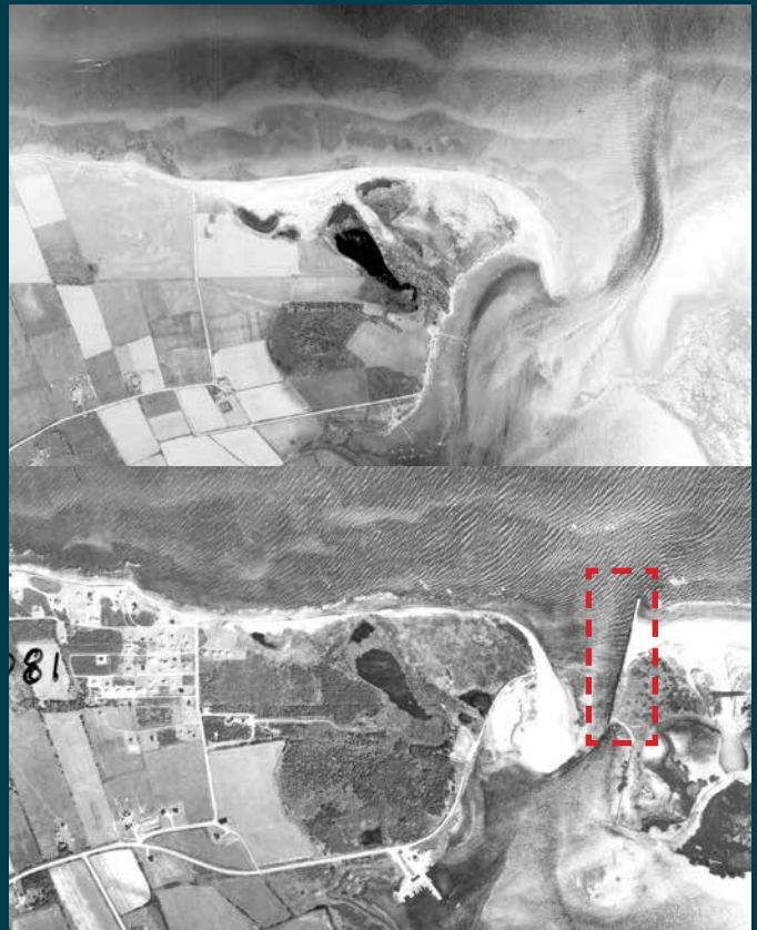
Figure 71. Comparison of the sandy beach conditions at Savage Harbour 1936 (before the breakwater) and 1990 (after). Breakwater outlined in red..
