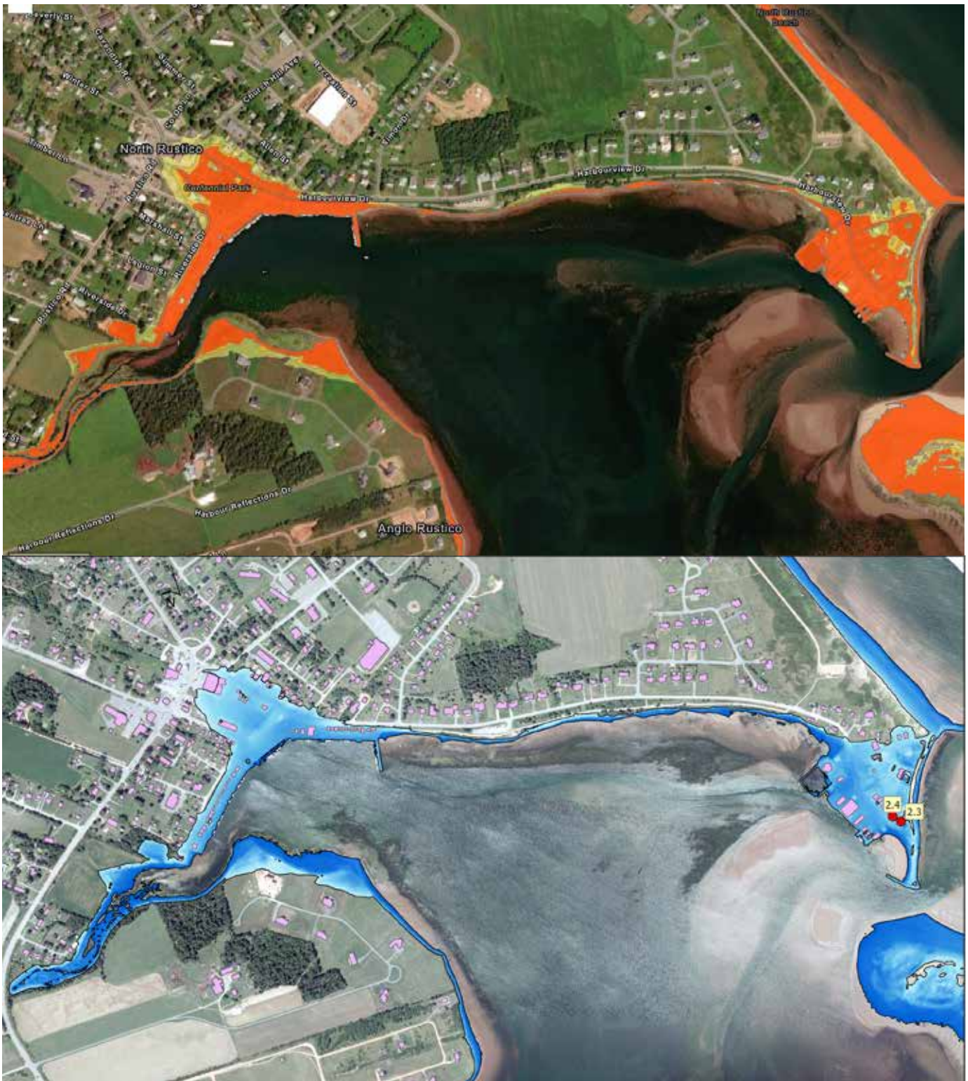
Figure 24. Top: Coastal floodplain (red) for North Rustico (Gov PEI, CHIP 2023). Bottom: Actual coastal flood extent (blue) following post-tropical storm Fiona based on high water mark survey elevations (Jardine, 2023a)
