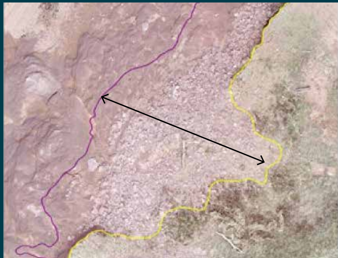
Figure 36. Drone orthomosaic for 2022 with coastlines comparing change over one year (purple is 2021, yellow is 2022) at Cape Gage showing a single point loss of about 17.5 m in a single year (UPEI, 2023)
