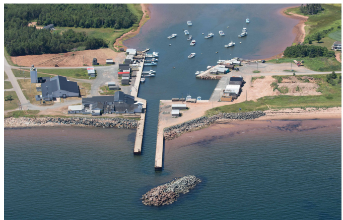
Figure 5. Graham's Pond Small Craft Harbour with shoreline armouring and offshore breakwater/reef (D. Jardine, 2023)
